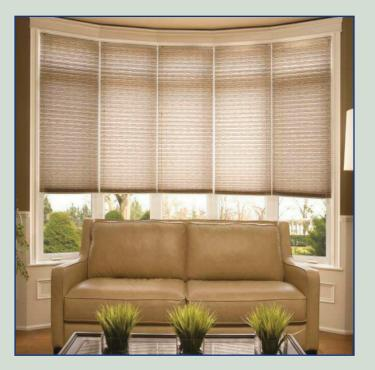
The main difference is a bay window sits on an area that protrudes from the normal elevation of the property, while with a bow, it is just the window itself that juts out.
